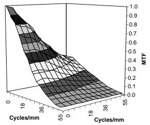
Figure 3. Section of the rotational MTF of the scanner after decimating by 20 points in both frequency directions.
